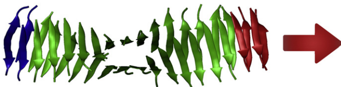
Fig. 2. Constraint schematic of hIAPP fibrils for fix-free constraint tensile loading simulation. Blue color means the fixed area and red area color means the pulled area.
